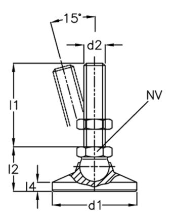
A/F = 15 d1 = 50 d2 = 10 l1 = 80 l2 = l4 = -Static load (N) = 11 Weight in (g) = 222
